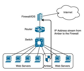
Figure 4.14: Amber architecture for a small network
