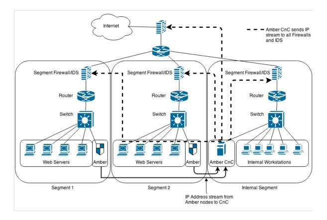
Figure 4.15: Amber architecure for a complex network with CnC server
