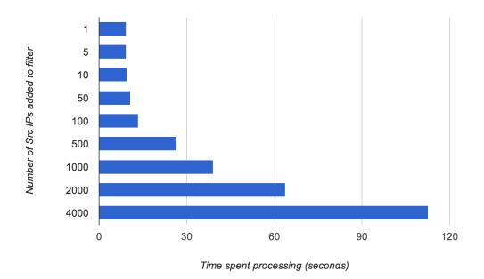
Figure 3.8: Processing time per IP (500mb pcap file)
